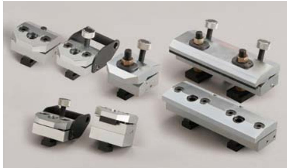
Use Ledge Clamps (Fixed Clamp Height Rocker Clamps) with dies having a clamp plate that sticks out from the die body or has a large slot.
