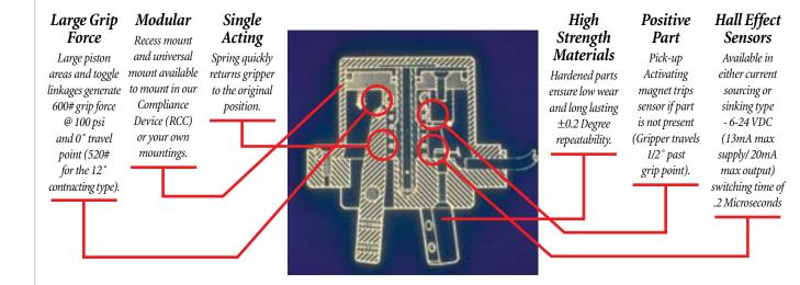
GTP grippers are designed to accommodate added tooling on the fingers and grip complex components using PFA's Gripper Pads (page 11). "3X" Style units are excellent for ID and Inside Bore applications and Recess Mount "R" style units mate easily with our Compliance Devices to support "jam free" assembly.
