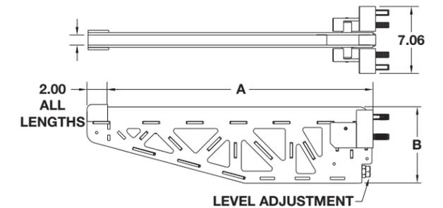
PFA recommends machining or shimming slots to 1.525”-1.530” for a die lift of approximate .060”.
