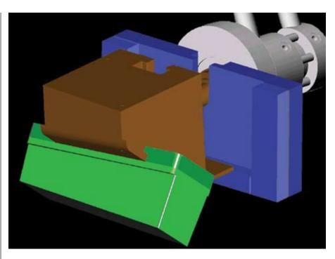
3-D of the mold slide with a preloading and locking cylinder style core system.
